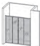
Alcove with sliding doors, available in 120-160 cm. Height 190 cm. Door opening 53-70 cm (see table). 4 & 6 mm hardened safety glass. Spring action door with eight ball bearings. Clamp mounting, no screws in the wall. Adjustable seal included. Delivery time: 2-3 weeks.
